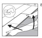
Lift the plank (together with the previous one laid in the same row) slightly up (about 30mm (1.2"), push it against the row in front and then put it down.
