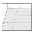
Lay the PE film, allowing at least 20cm (8") of overlap and use adhesive tape to unite. Turn the film upwards 5cm (2") along the walls
